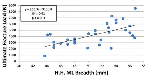
**A2. Ultimate Fracture Load vs. Humeral Head ML Breadth**
