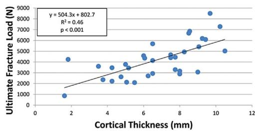
**B2. Ultimate Fracture Load vs. Combined Mean Cortical thickness at D3**
