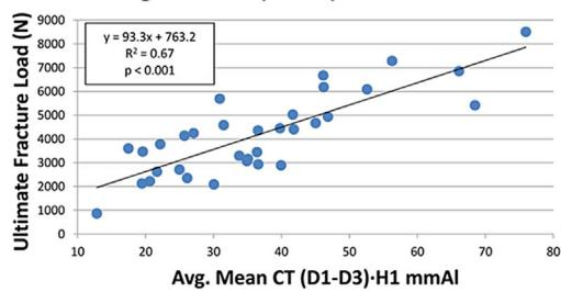
**D2. Ultimate Fracture Load vs. Avg. Mean CT (D1-D3)·H1 mmAl**
