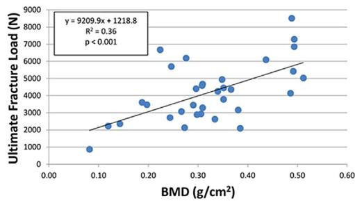
**C2. Ultimate Fracture Load vs. BMD**
