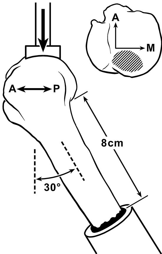
**Figure 2.** (A) Diagram of a loaded left humerus in lateral view; A = anterior; P = posterior. (B) View of the superior humeral head showing the area (oblique lines) where the force was applied to the humeral head; A = anterior; M = medial.
